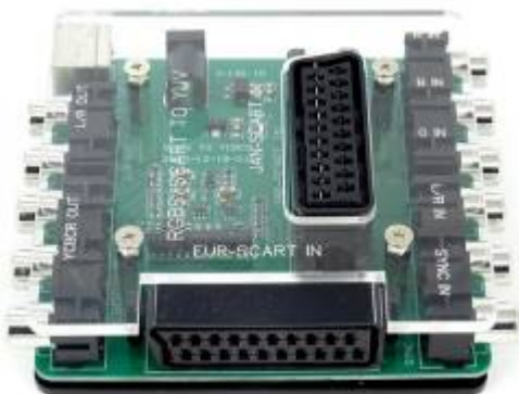
Convert VGA to Scart cable to YCBCR & S-Video
