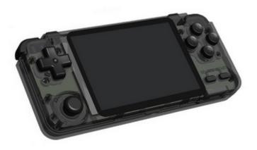
Basically a pre-assembled version of the Odroid Go Advance. Some would say a "clone". First production units had a battery issue, but this was resolved in later manufacturing runs. Build quality is kind of crummy (visible seams, no passive heatsink) but is slightly better than that of the Odroid Go Advance. The plastic shell comes in translucent indigo or translucent black. The metal shell comes in black.
