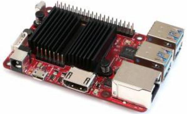
A mid-priced \$54 USD board. The current version of the Odroid C line of SBCs. Could be considered of the same generation as the Pi 4. Uses a more powerful amlogic S905gen3 ARM CPU. Good for a wide range of emulators.
