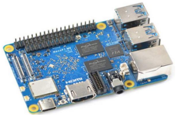
A mid-range \$70 board. The NanoPi M4V2 is powered by the Rockchip RK3399 ARM CPU.
