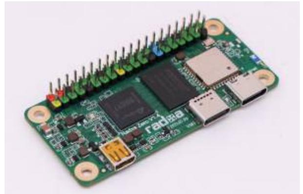
A cheap \$35 board. The [Radxa Zero](#) is a small form-factor board similar in shape to the Raspberry Pi Zero, but significantly more powerful (powered by the s905gen2 SOC). Support for this board was introduced in Batocera **v32**. Supports models
