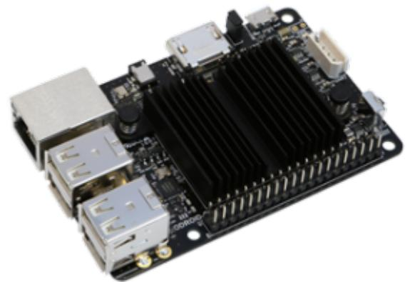
Odroid C line is similar to the Pi in terms of being an SBC the size of a credit-card, but has a slightly better amlogic S905 ARM CPU. The C2 could be considered of the same generation as the Pi 3. This device is discontinued, replaced by the C4. With that said, still good for a wide range of emulators.
