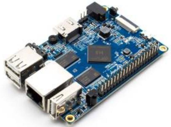
Cheap \$30 board. The [Orange Pi PC](#) is powered by the AllWinner H3 CPU clocked at up to 1.6GHz. A customized, downgraded version of this board is used in the [Capcom Home Arcade](#). Successor to the similarly spec'd Orange Pi One.
