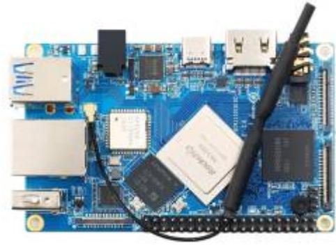
A modestly-priced \$50 board, one of the main competitors against the Raspberry Pi. The Orange Pi 4 is powered by the RK3399 SoC clocked at up to 2.0 GHz, its more powerful than the RPi 4 while being cheaper.<sup>2)</sup>
