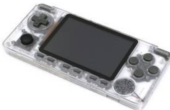
Mid-to-high priced; \$60 USD for the Advance, \$80 for the Super. Based on the RK3326 ARM CPU, this is a portable handheld gaming system.
