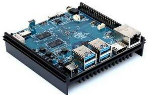
A mid-priced \$66 USD board. Powered by the Amlogic S922X ARM CPU! Even if it's a bit larger than a Raspberry Pi, it's still very small for bartop/arcade projects. It's also much more powerful while still being completely fanless. Compared to a Raspberry Pi, the Odroid N2/N2+ doesn't provide Wi-Fi or Bluetooth out of the box (but many USB Wi-Fi and/or BT dongles are compatible).
