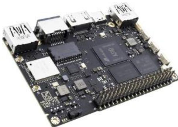
[Khadas VIM3](#) has a powerful Amlogic A311D SoC: x4 Cortex A73 performance-cores (2.2Ghz), and x2 Cortex A53 efficiency-cores (1.8Ghz) are merged into a hexa-core configuration, and fabricated with a 12nm process to maximise performance, thermal and electrical efficiency. Support introduced in Batocera.linux **5.27**.
