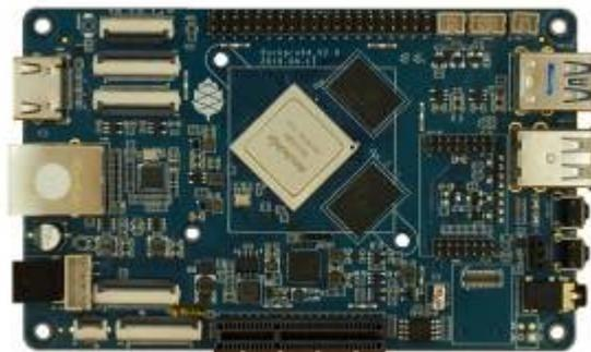
A mid-ranged priced \$60 USD board. The [ROCKPro64](#) is powered by the Rockchip RK3399 Hexa-Core (dual ARM Cortex A72 and quad ARM Cortex A53) 64-bit CPU with the MALI T-860 Quad-Core GPU. This is the most powerful SBC offered by PINE64 as of writing.
