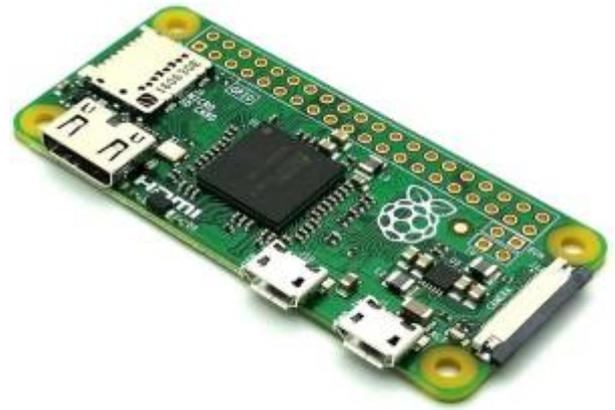
A cheap \$5 USD board. Single core ARM processor clocked at 1 GHz with 512 MB DDR2 Ram. The W/WH model has Wireless and Bluetooth built in. This version of the Pi has been continually refreshed throughout the lifespan of the other Pi devices, the first iteration was identical to the Pi 1's specifications at 700MHz, whereas the current ones being manufactured have an upgraded 1 GHz CPU. The Pi Zero is a popular choice when used in conjunction with a [Retroflag GPI Case](#) for handheld emulation.
