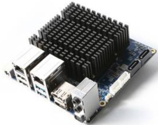
High-priced \$120 USD board. Technically an ordinary x86 machine, powered by Intel UHD 600 integrated graphics. Pretty large compared to other SBCs. Should work with Batocera's 64-bit build, but testing needs to be done.
