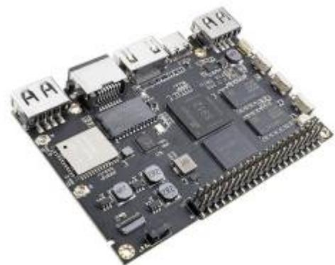
**Khadas VIM2** has a beefy Amlogic S912 SoC: x4 Cortex A53 performance-cores (1.5Ghz), and x4 Cortex A53 efficiency-cores (1.0Ghz) are merged into a octo-core configuration, coupled with a Mali-T820 MP3 GPU running at 600 MHz. Support was introduced in Batocera.linux **29**.
