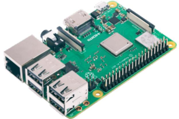
Cheap \$35 USD board. The most “mainstream” Raspberry Pi available still in manufacture. Recommended to get the B+ model. You'll find most accessories/HATs/cases are only compatible with this model or lower, and is probably the easiest Raspberry Pi to find/source as of 2020. The original B model had pretty poor Wi-Fi/Bluetooth reception, but this was fixed in the B+ model.
