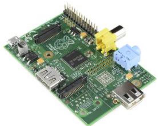
A cheap \$30 USD board. The original model of the first Raspberry Pi. Basically the same specs as Pi Zero but clocked at 700Mhz. Recommended to get the B model. This board has gone through multiple revisions but the newest looks identical to later B models with the 4 USB ports. Considered discontinued, though new models are still being manufactured. Look into the newer Pi3 or Pi4 models for better emulation performance at a similar price.
