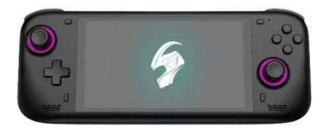
Ayn Lokis are x86\_64 handhelds (while Odin are ARM-based). An Ayn Loki is sold with Windows 11, but it also supports the regular x86\_64 Batocera image and can be booted on the SDCard port.
