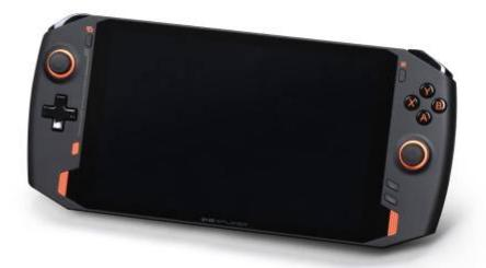
The OneXPlayer (Intel Tiger Lake i5 or i7 11xxG7 CPU, with a 8.4" screen) is supported out-of-the-box with Batocera **v32** and later versions. The OneXPlayer S1 should also be supported, but has yet to be tested.
