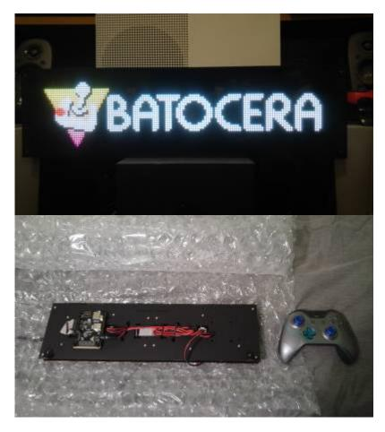
This is the lower resolution LED panel that's more suited to pixel-art display than full-color images. It's easy to tell this one from the LCD panel as it has a USB port on the back, while the LCD panel does not. This panel comes in two sizes, pictured above is the smaller size next to an Xbox One controller.
