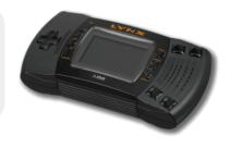
It has a WDC 65SC02 CPU. Notably, it was the world's first handheld system that used a color LCD screen, as well as having fairly advanced graphics for the time. It featured buttons on the top and bottom of the right side of the unit, allowing games to be played in either sideways landscape mode, or upright portrait mode.
