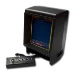
The Vectrex features an integrated monochrome CRT monitor, but this isn't just any CRT monitor that scans left-to-right, top-to-bottom. Instead, the electron beam is able to shoot freely across the face of the entire phosphor screen, from any angle, up to the length of the monitor. In essence, this is producing vector graphics as they are literally being generated on the machine. To this date, the Vectrex is the only vector display-based console released for the home market ever.
